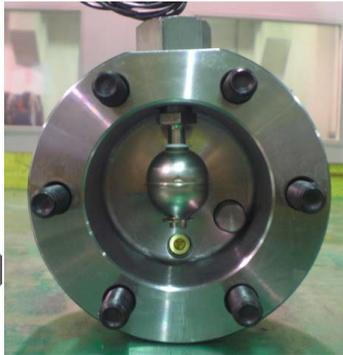
Photo shows assemble with 'O Rings' Vibration Shield and gaskets in place.
