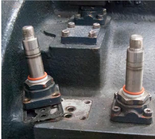
Step 1 - Remove Load Solenoid and Gasket
